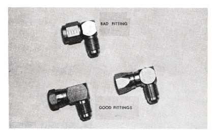
Please notice the difference in the nut style of the defective adapter and the good adapter. Destroy all defective adapters in inventory and submit a warranty request for compensation.
